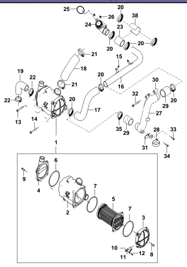
**36**: SET\_PIPE\_INTERCOOLER, INLET (20+27+28+29+32+34+35)
