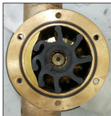
<Seawater pump & Impeller>
