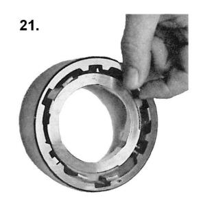
Fit the tension rollers on the shafts for suspension by rollers.
