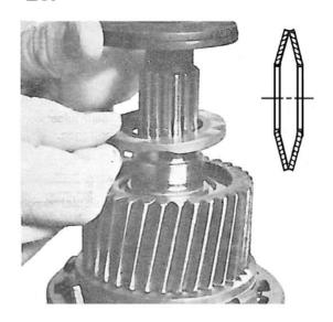
Check the tightening of the disc springs.
