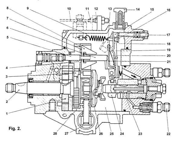
The centrifugal governor is placed in the upper part of the fuel pump.
