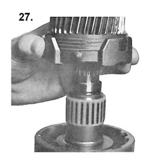
Fit thrust washer, the oil pockets of which should turn towards the wheel for "AHEAD".
