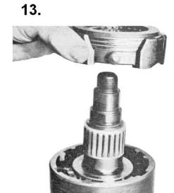
Remove the wheel "AHEAD" with a special tool and take off all parts "AHEAD".
