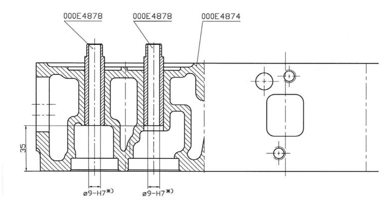
\*) The valve guides tolerance after fitting
