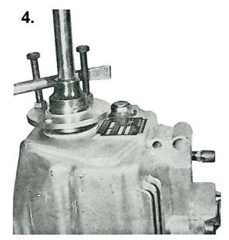
Pull off the output shaft flange.
