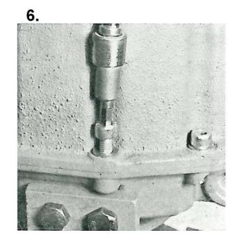
Drive back the fitting pins 2-3 mm in the gearbox and lift one gearbox half with reversing shaft, input and output shafts free of the other gearbox half.
