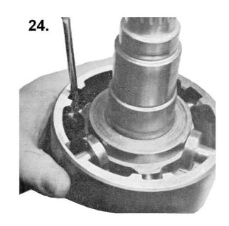
Fit needle bearing housing, wheel for "AHEAD" and washer.
