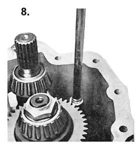
Lift the complete arrangement with input and output shafts and shifting fork out of the housing.
