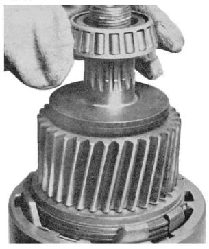
"Note": Fix the tapered roller bearing for "ASTERN" with supporting washer and original hexagon nut.
