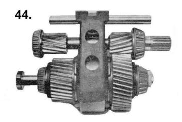
Fit the intermediate wheel and needle bearing.
