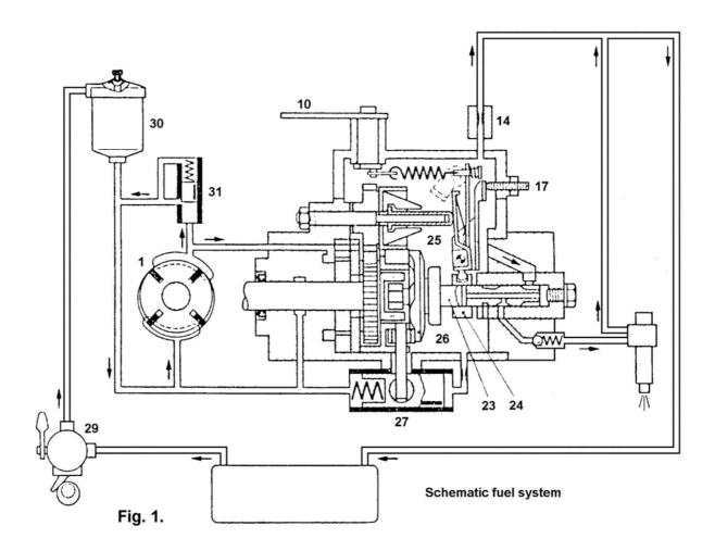
Through the pressure control valve (31), after the feed pump, a pressure is produced. Most of the fuel flows through the pressure control valve back to the suction side. The remaining part of the fuel flows through the inner chamber of the pump (fuel chamber) (25) to the high pressure chamber of the distributor head and then it is led to cooling and bleeding and then back to the tank through the overflow throttle (14).
