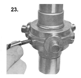
Press the sliding sleeve from the bottom against the check bolts.
