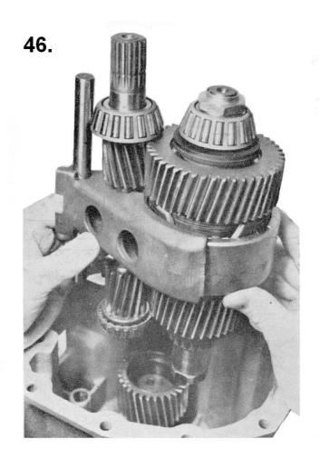
Fit retaining plate for intermediate wheel and before that smear the screws M8x25 with Loctite No. 241.
