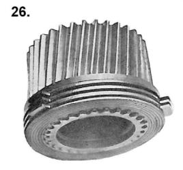
Fit wheel for "AHEAD" with clutch discs on the thrust collar.
