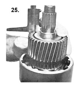
First fit a washer. Then fit an inner disc and the an outer disc.
