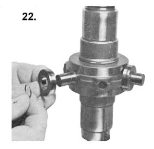
Fit the pressure springs in the check bolts. Fit the check bolts in the corresponding bores.
