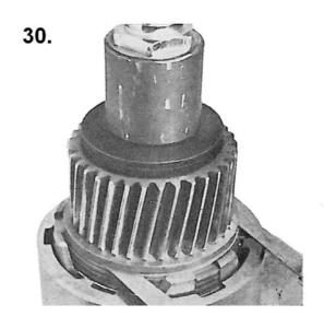
Heat the tapered roller bearing inner collar to about 85°C and fit it with the thin end of the taper roller facing the shaft end of the output shaft until it fits tightly against the disc springs.
