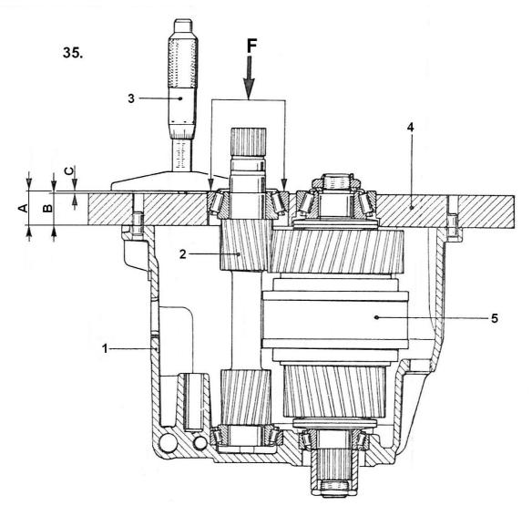
1 = Housing 2 = Input shaft 3 = Depth micrometer
