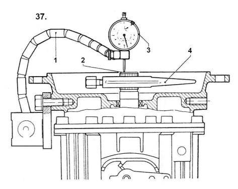
1 = Dial indicator holder 2 = Input shaft 3 = Dial indicator 4 = Driving arrangement
