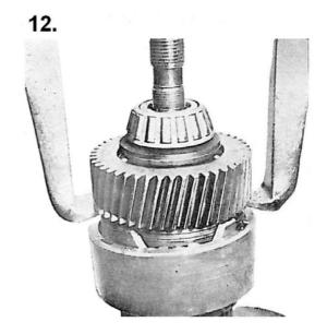
Remove the thrust collar wuth bolts and washers together wuth needle bearing bushing, sliding sleeve and pressure spring.
