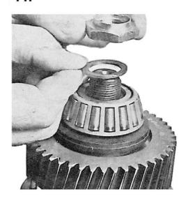
Pull off the wheel "ASTERN" with a special tool and take up washer, disc springs and tapered roller bearing inner collar.
