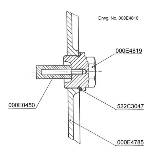
It is not necessary to exchange the plug as the zinc anode is screwed on to this.
