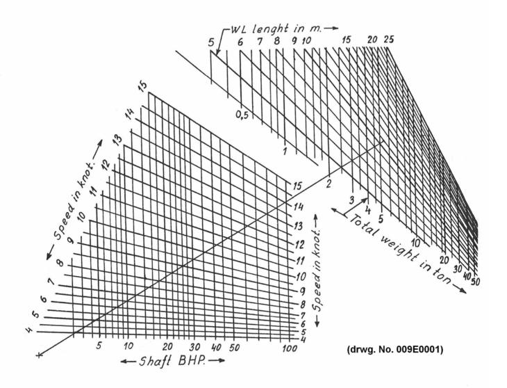
Seek the scheme to the right of the intersection between the actual length in the waterline of the ship and the total weight.
