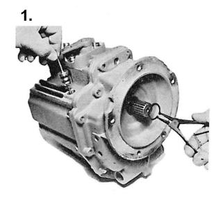
Remove the shifting arrangement with gasket.
