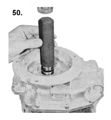
Smear the similar seal ring 32 x 45 x 7 for the output shaft in the same way as the seal ring for the input shaft and fit it by means of punch No. 1 x 56 136 993 in the housing so that it fits tightly against the tapered roller bearing inner collar.
