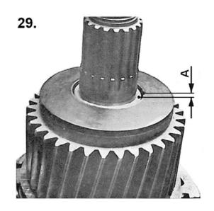
Tighten the disc springs with bush 1 x 56 136 994. Measure disc clearance between inner disc and washer with a feeler gauge in two places which are opposite one another.
