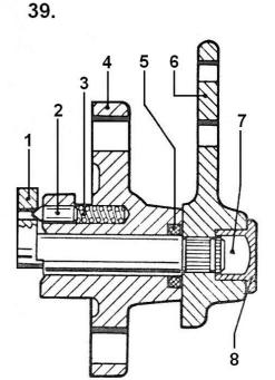
Press the shift control lever on to theshifter shaft so that shift control leveris placed in neutral position at 90°±30'to the gear shaft length.
