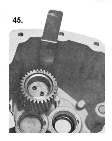
Place the housing so that the opening of it turns upwards.
