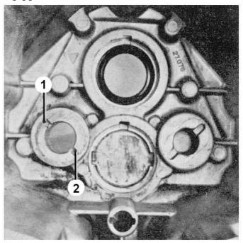
Heat the gearbox and fit the bolts with slotted pins in pos. 1 or 2 all depending on the transmission.
