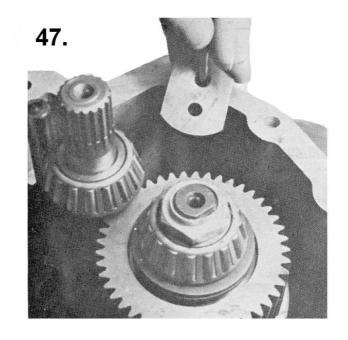
Smear the seal f aces of the gearbox halves wit h permanently plastic liquid jointing.
