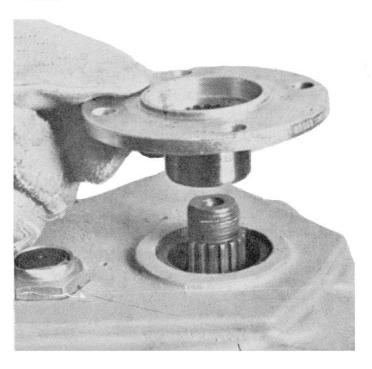
Smear the nut with permanently plastic liquid jointing and secure it with a torque of 100 Nm ( 10 Kpm).
