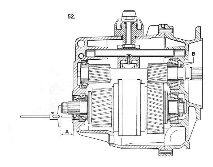
A = Distance to shaft seal ring:  $22.5 \pm 0.5$  mm.
