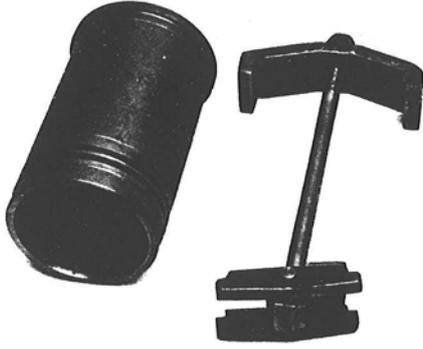
Puller for cylinder liner
