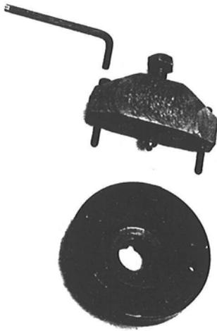
Puller for flexible coupling
