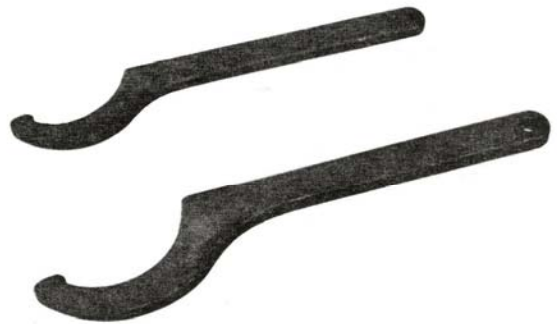
SKF hook spanner HN10 and HN12 for nuts on crank Order Nos. 60680 and 60681
